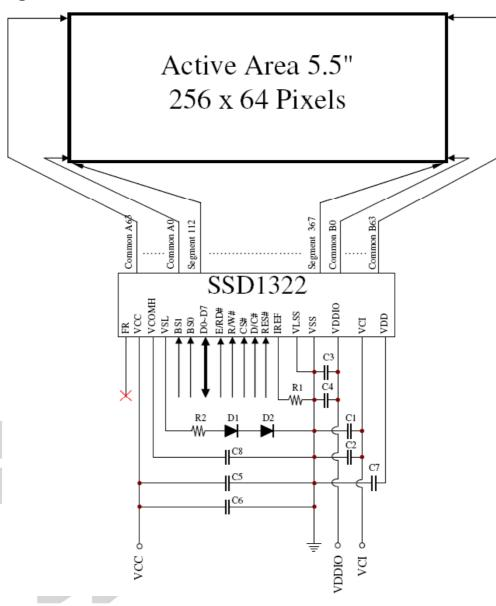
$\begin{array}{cccc} \text{C1, C3, C5} & :0.1\,\mu\,\text{F} \\ \text{C2, C4} & :4.7\,\mu\,\text{F} \\ \text{C6} & :20\,\mu\,\text{F} \\ \text{C7} & :1\,\mu\,\text{F} \\ \end{array}$
